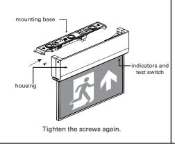
Step 8: Switch the mains supply on.
