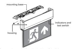
Remove the screws from both sides of the light to separate the mounting plate from the luminaire.
