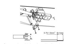
Secure mains cable by using cable clip and screws.
