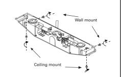
Drill where indicated and use wall plugs and screws, to fix the housing in the desired position.
